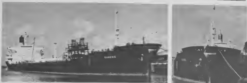
The tanker to bring a record crude cargo to Lago was the "Eugenie". With a length of 774 feet, 105 feet beam and 64,000 deadweight tons, the Liberian tanker carried 375,000 barrels of crude from Maracaibo to San Nicolas Harbor on February 14.
